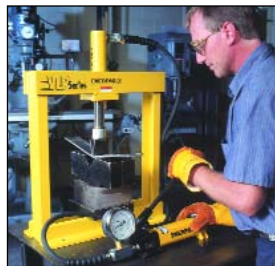
◀ VLP-Series 10 ton bench press, used in this maintenance workshop to bend steel flat bar.
